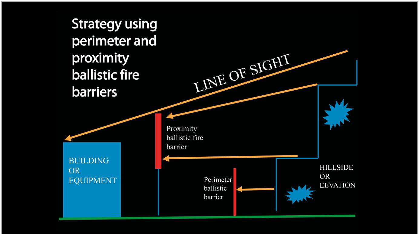
Figure 7. Using proximity/perimeter barriers for Line of Sight compliance
